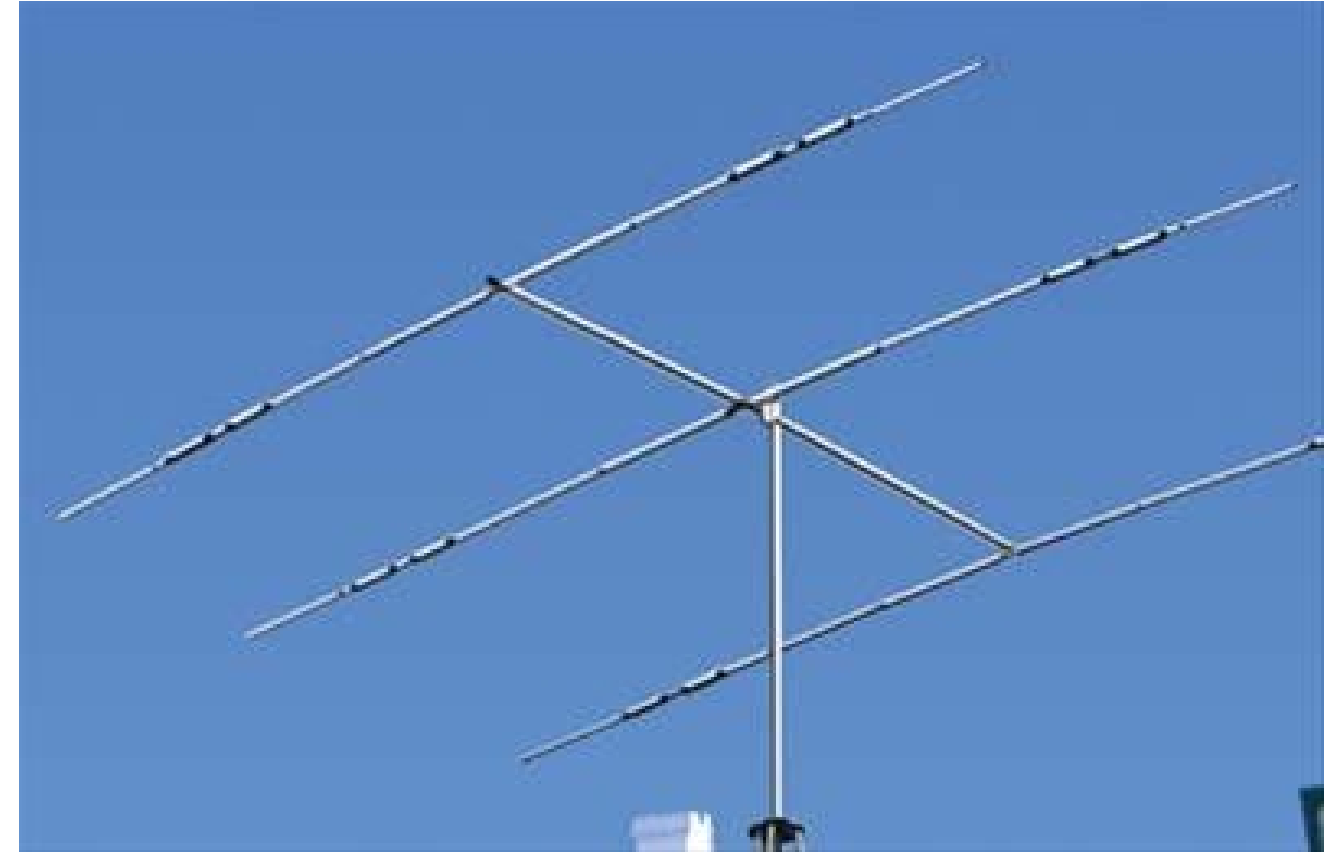
Yagi Arrays - dipoles with reflectors and directors
